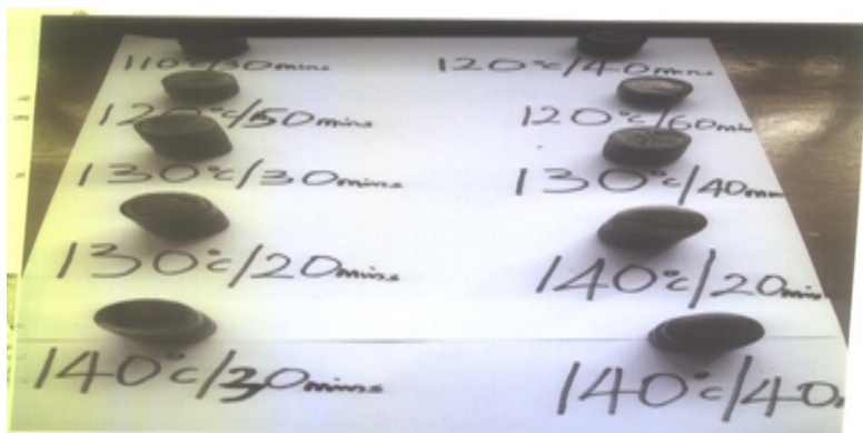
Fig. 30b Polyethylene Wax Produced from Pure Water Sachets Showing Pyrolysis Temperature and Time (Source: Ademiluyi, Obobo & Akpan , 2013)
