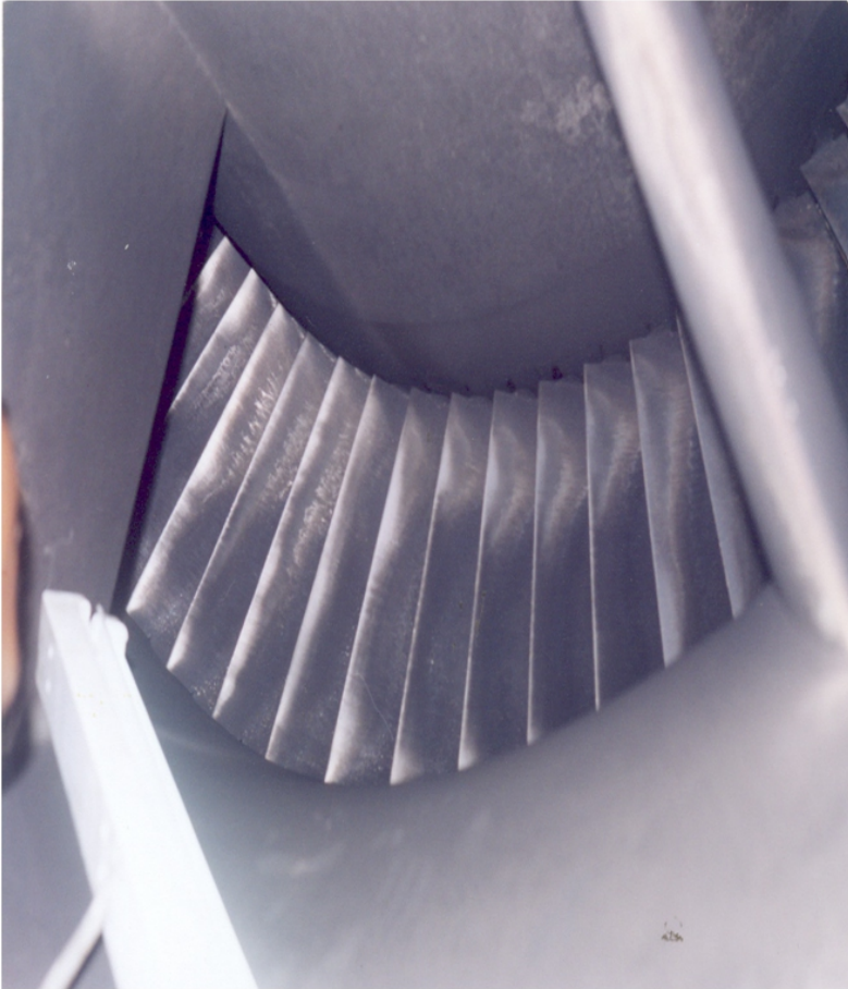
Plate 2: A Second View of Contaminated Compressor Blades
