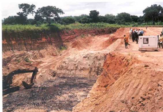
Plate 1: Open cast coal mine at Okaba, Kwara State (Photo by Eze, C.L, 2022).
