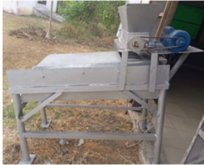
Plate 4. The gari sifting machine
