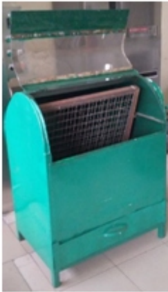
Plate A3: The plantain, yam and fish roasting machine
