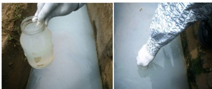
Plate 10: Collection of samples at the Midstream flow of effluents from the company
