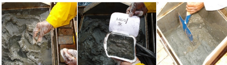
Plate 6: Subsampling of sediment for microbiology, physicochemical and macrobenthic analysis
